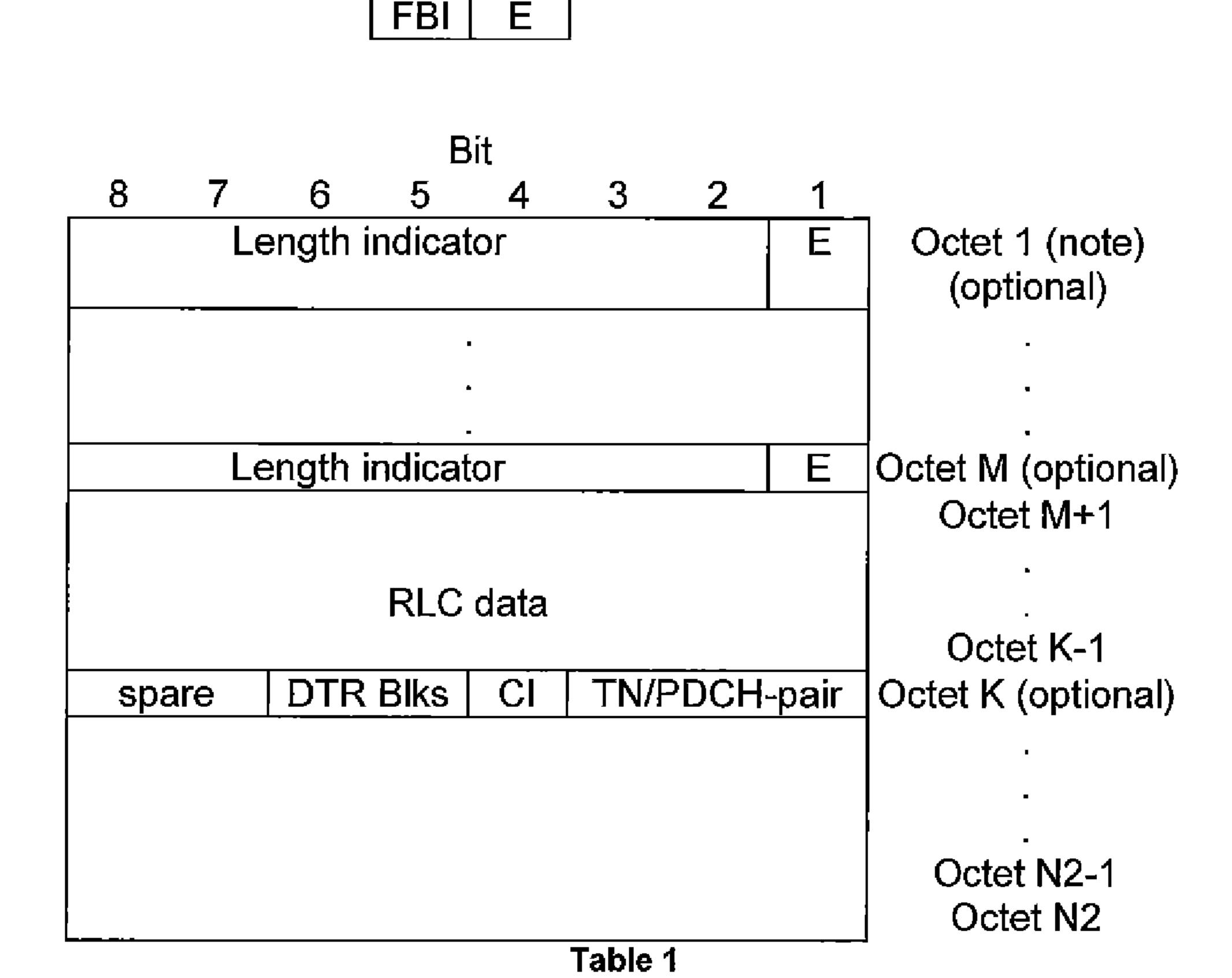
[0023] Referring to Table 1, the carrier ID (CI) field contains a identification of the carrier that may be encoded as DTR\_CI IE. The CI field can be used to indicate the carrier that the MS monitors when DTR is used. In that case, the timeslot or PDCH-pair to monitor on that carrier can be indicated with the TN/PDCH-pair field.
