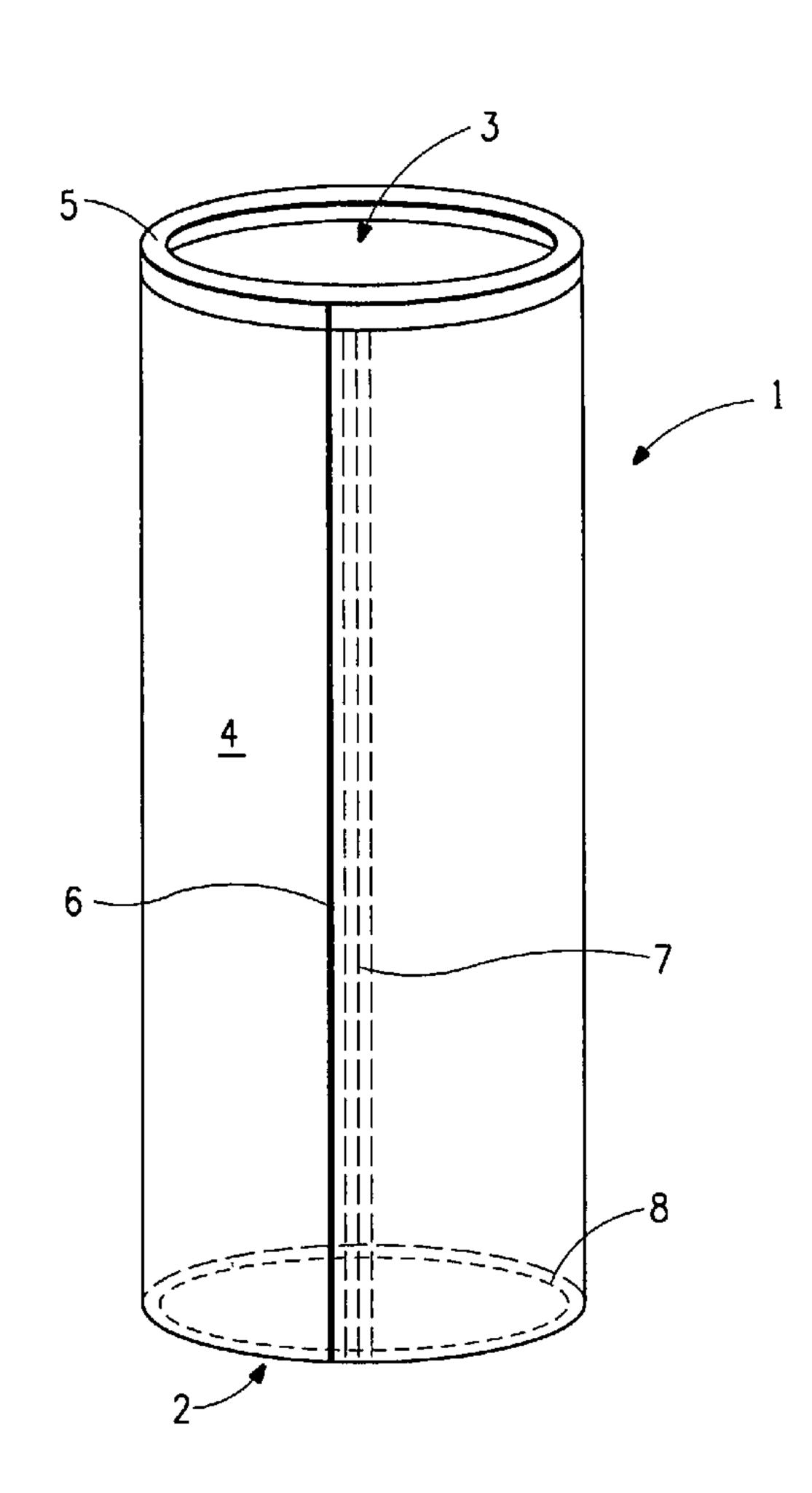
(57) Abstract: This invention relates to a bag filter having a tubular section, one closed end and one open end, the tubular section having a nonwoven felt comprising an intimate fiber blend of 50 to 80 parts by weight meta-aramid fiber and 20 to 50 parts by weight acrylic fiber, based on the total weight of meta-aramid and acrylic fibers in the felt, wherein the acrylic fiber has an equal or lower denier per filament than the meta-aramid fiber.
