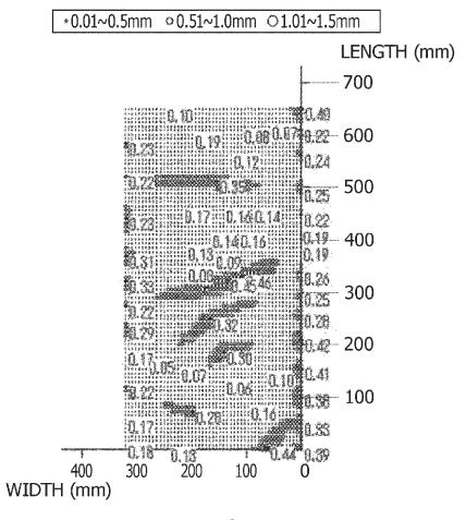
\* SIZES OF BUBBLES () INDICATE AMOUNTS OF LIFT OF RESPECTIVE PORTIONS FROM HORIZONTAL SURFACE PLATE NUMERICAL VALUES IN GRAPH INDICATE LIFT HEIGHTS
