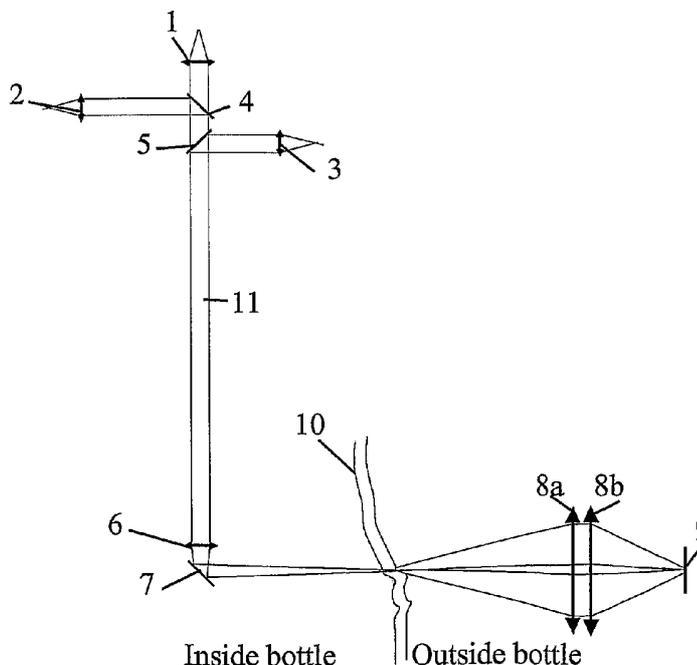
(57) Abstract: The present invention is related to an apparatus and a method for measuring the coating thickness deposited inside or outside a plastic container by measuring the internal transmission at two wavelengths. One wavelength is in the infrared range, i.e. longer than 750nm, and allows to subtract the absorption of the substrate while the other wavelength is shorter and chosen in a range wherein absorption by the coating is maximum and absorption by the substrate is moderate.
