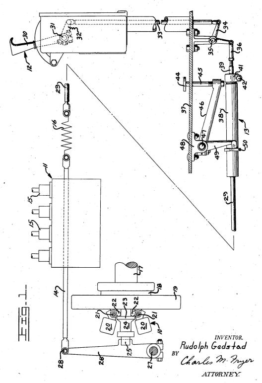
AUXILIARY DECELERATOR FOR INTERNAL-COMBUSTION ENGINES
