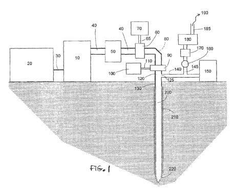
(57) Abstract: System for drilling boreholes into subsurface formations. A gyrotron injects millimeter-wave radiation energy into the borehole and pressurization apparatus is provided for pressurizing the borehole whereby a thermal melt front at the end of the borehole propagates into the subsurface formations. In another aspect, a system for fracturing a subsurface formation is disclosed.
