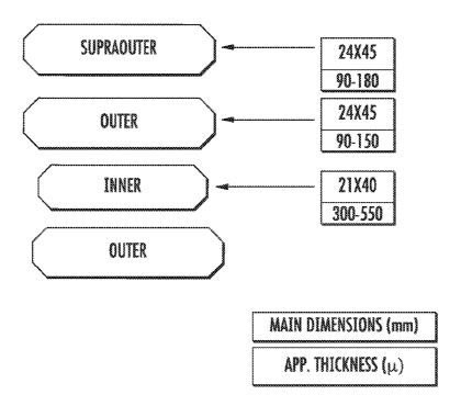
A SCHEMATIC DRAWING OF THE FILM COMPONENTS OF A GRDF WITH AN IMMEDIATE RELEASE LAYER AND THEIR APPROXIMATE DIMENSIONS
