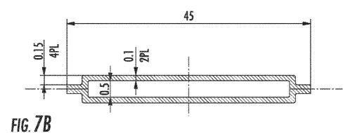
A DRAWING OF THE ULTRASOUND WELDING ON THE GRDF (A).
