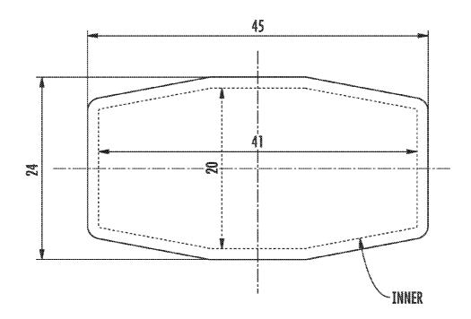
A DRAWING OF THE CURRENT GRDF DESIGN SHOWING THE PLANAR DIMENSIONS OF THE WHOLE GRDF AND OF THE INNER LAYER
