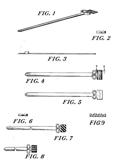
FIG. 1 is a front perspective view of a bundling strap showing my new design;
