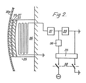
This invention relates to aircraft de-icers and more particularly to electrical impulse de-icers suitable for de-icing thin walled aircraft structures and gas turbine engine parts.
