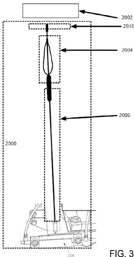
(57) Abstract: The present example provides an automated or mechanized, way of making a pepper boat from a de-stemmed pepper. In making the pepper boat, de-stemmed peppers may be split by a splitting assembly. As the pepper is split, or subsequently, a whisk assembly tends to clean a portion of the veins and seeds from the split pepper pod to form two substantially equal halves of a pepper boat, suitable for further food processing.
