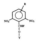
where R is not critical provided it is neither acidic nor absorbs sufficient UV exposing light to substantially decrease sensitivity. Exemplary substituents for R are H, lower alkyl and halogen (all R's need not be the same). R' is advantageously H or  $CH_3$ , while Y is preferably reactor was maintained in quenched by cooling to 0° mately 100 mL of acetone. The resulting terpolymer tion medium by adding this
