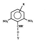
where R is not acidic, R' comprises a member of the group consisting of H and  $CH_3$  and Y is chosen so that it requires a temperature of at least 75° C. to cause its removal from the remainder of said photosensitive acid generator.
