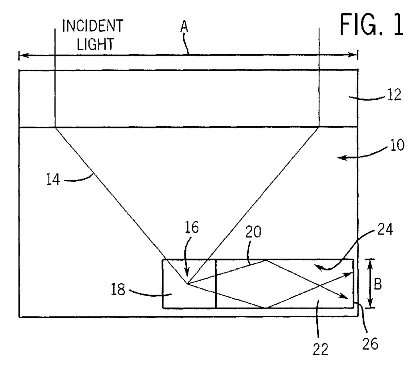
(57) Abstract: An optical concentrator having a concentrating element for collecting input light, a redirecting element for receiving the light and also for redirecting the light, and a waveguide including a plurality of incremental portions enabling collection and concentration of the light onto a receiver. Other systems replace the receiver by a light source so the optics can provide illumination.
