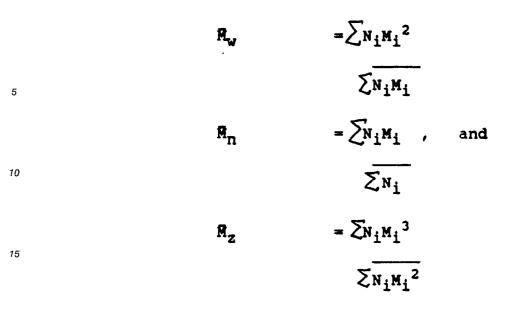
wherein N<sub>i</sub> is the number of molecules of molecular weight M<sub>i</sub>. 20 d. Viscosity Index (V.I.) is the ability of a lubricating oil to accommodate increases in temperature with a minimum decrease in viscosity. The greater this ability, the higher the V.I. Viscosity Index is determined
