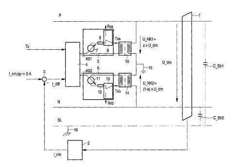
(57) Abstract: In a wire-bound network which comprises unshielded lines such as power supply lines, electromagnetic radiation is produced when transmitting data above the mains frequency. The device according to the invention comprises active means for reducing or eliminating the common-mode current (I-cm). To this end, these active means generate an artificial dissymmetry which is complementary to that of the network and is measured continuously or periodically.
