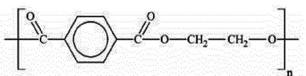
**[0006]** Terephthalic acid (PTA) and ethylene glycol (EG) are esterified and polycondensed to produce PET melt; PET melt is then underwater pelletized to produce PET masterbatch, and then to spin.
