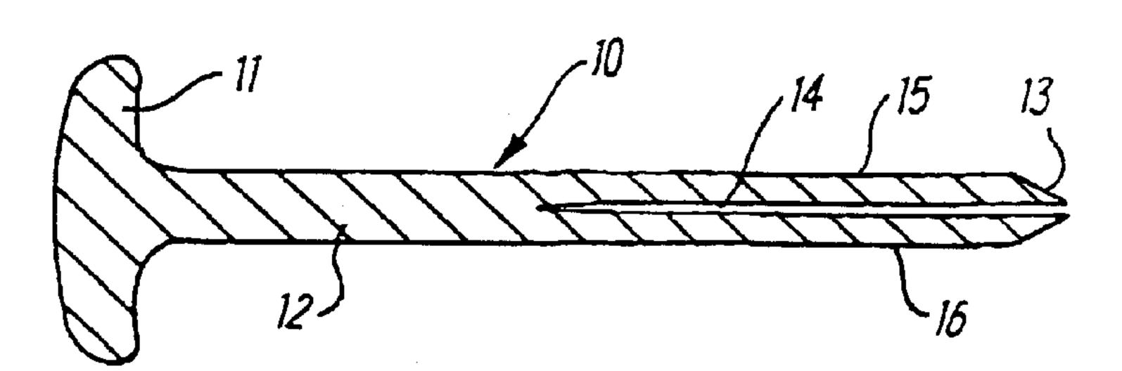
(57) The edge 17 of a filter cloth 18 is received in a slot 14 formed in an edge 13 of a planar part 12 of an edge strip 10, extending parallel to and preferably lying in the axis of the plane of said planar pan 12. The edge strip also comprises a track portion 11 defining its outer edge and formed integrally with the planar part 12. The slot 14 may be formed by use of a hot air knife or by a metal blade and defines upper and lower flaps 15,16 which are adhered to the edge 17 of the cloth.
