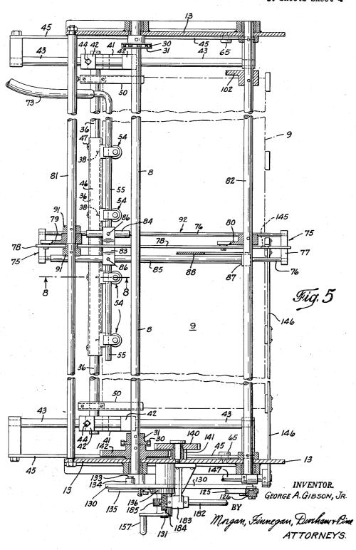
G. A. GIBSON, JR APPARATUS FOR FEEDING, CUTTING AND STACKING FLAT STOCK
