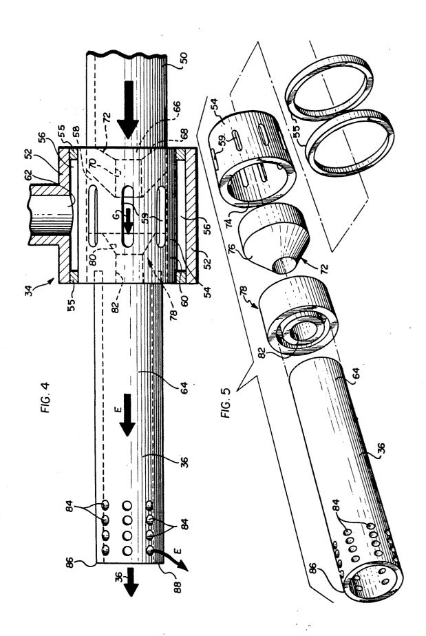
HIGH PRESSURE OXYGEN-SATURATED WATER-TREATMENT
