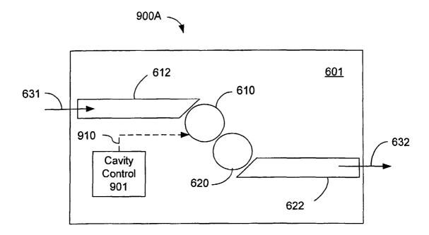
(57) Abstract: Optical filters (900A) having at least two coupled whispering-gallery-mode (WGM) optical resonators (610, 620) to produce a second order or higher order filter function with a desired spectral profile. At least one of the coupled WGM optical resonators (610, 620) may be tunable by a control signal to adjust the filtering function.
