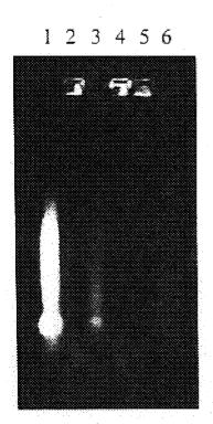
**Figure 3.** Recovery of rRNA after electrophoresis at pH 2.5 in Gene*CAPSULE*. A 1% agarose gel was prepared and run in TBE, as described in the text. Lane 1. 1 ug each of 23 S. 16 S. & 5 S rRNA; lanes 2-6 equal proportions of fractions from Gene*CAPSULE*, as listed in Table 1.
