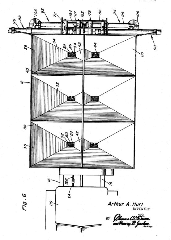
FERTILIZER MIXING AND SPREADING MACHINE
