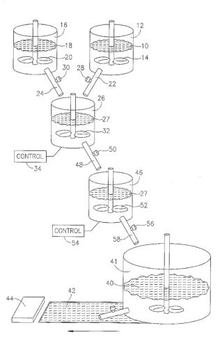
(57) Abstract: A method including improving a property of a paper product precursor by adding a molten-wax suspension to a slurry including the paper product precursor, the molten wax suspension including a suspension of molten wax particles in a liquid solvent, the liquid wax particles being at a temperature higher than the melting point of the wax.
