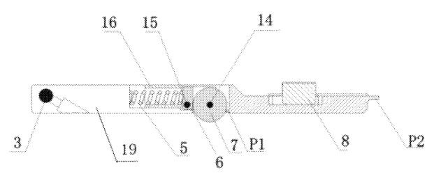
According to the anti-rotating device of the non-rotating sleeve and a rotary guiding device, on the one hand, bases can be provided for accurate attitude measurement and guiding control, on the other hand, excessively rapid rotation of the two non-rotating sleeve can be prevented only by using one anti-rotating device, and meanwhile the antirotating device can further provide guiding driving force based on the minimum structure size.
