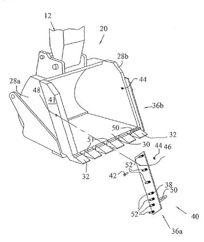
(57) Abstract: An apparatus (36) coupled to an excavation bucket (20) for creating a trench (24) sidewall (28) having indentations (34) formed therein.
