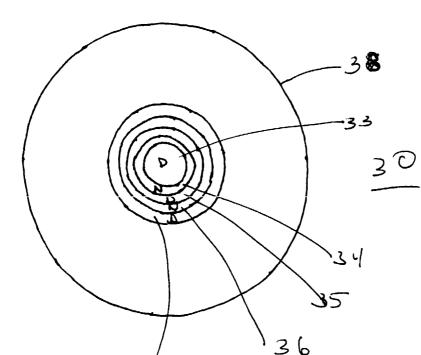
(57) Abstract: The invention provides multifocal ophthalmic lenses that have zones of more than one optical power, or focal length. The lenses correct for high order optical aberrations in more than one field of gaze.
