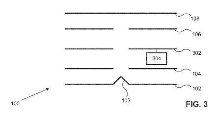
(57) Abstract: A field emission device is configured as a heat engine, wherein the configuration of the heat engine is variable as a function of time.
