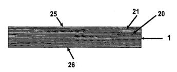
(57) Abstract: The present invention provides a stretchable material suitable for use in an inflatable medical device. The stretchable material has at least one reinforcing polymer layer with a top and bottom side forming a porous matrix which is imbibed with a sealing material to infiltrate and substantially seal spaces of the porous matrix and extend beyond the reinforcing polymer layer to form a surface coating.
