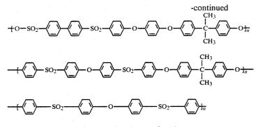
The above polysulfone portion has preferably a reduced viscosity  $[\eta_{sp}/C]$  in the range of 0.05 to 1.0, said reduced viscosity being a value calculated by the following equation from a relative viscosity measured at 25° C. for a solution of a polymer in chloroform in a polymer concetration of 0.2 g/100 ml. 20
