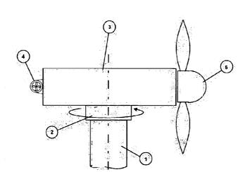
(57) Abstract: A water current generating device consisting of a main body (3) and a horizontal axis rotor (5) is attached by a mechanical connection (2) to a fixed support structure (1). Under the action of one or more hydrodynamic thrusters (4) the main body of the turbine is rotated about a desired axis of rotation to face the oncoming current flow. The mechanical connection incorporates an appropriate degree of freedom to allow this re-orientation to take place.
