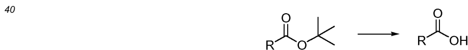
Scheme 69: TFA-mediated conversion of an ester to a carboxylic acid (General Procedure QQQ)
