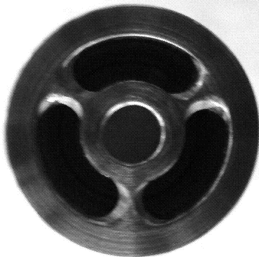
Figure 16: Outside View of Retaining Screen of Backflow Preventer Insert Valve
