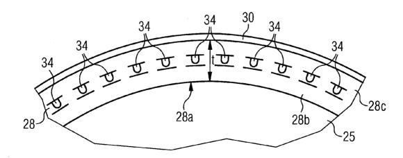
(57) Abstract: An imaging magnet having a patient bore (25) for receiving a human or animal patient, comprising a body coil assembly (24) comprising a body coil former (28) and a body coil (30). The body coil assembly is provided with at least one source of light (34, 36) incorporated within the body coil assembly for providing light into the patient bore (25).
