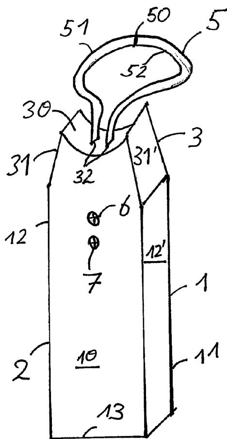
(57) Abstract: The invention relates to a device for determining measurements of human body parts (B), in particular leg and hip measurements which are to be determined for supplying compression tights, on which first measuring means (5), for measuring the peripheral length of said body parts (B), are provided. Said device also comprises second measuring means (6, 7) which can determine the longitudinal section (C) from the body part (B) on a reference plane to the peripheral plane (U).
