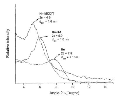
(57) Abstract: This invention relates to hybrid clays for obtaining nanocomposites useful in the automotive, aviation, construction and packaging industry, among others. The hybrid clay comprises clays intercalated with the itaconic acid (ITA) monomer or its derivative monoctadecyl itaconate (MODIT). The invention further relates to a process for the preparation of these hybrid clays and the process to obtain polyolef in/clay nanocomposites.
