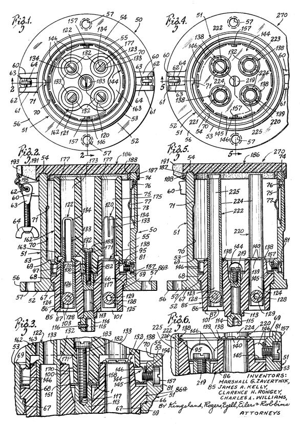
M. G. ZAVERTNIK ETAL ELECTRIC PLUG OR RECEPTACLE ASSEMBLY WITH INTERCHANGEABLE PARTS
