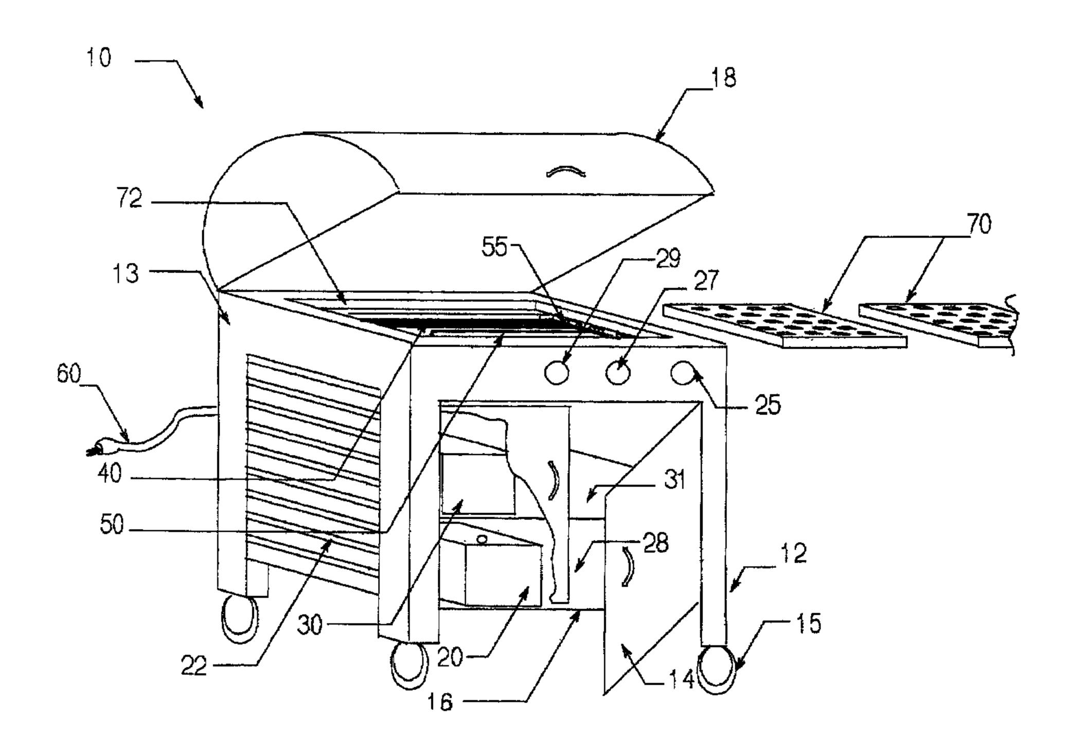
(57) The invention is a dual power source high heat electrical grill whose primary application is as an outdoor or indoor grill which uses the combination of AC and DC powered elements in a hybrid configuration to produce as much heat as conventional outdoor gas grills and more than could otherwise be produced by a conventional electric grill.
