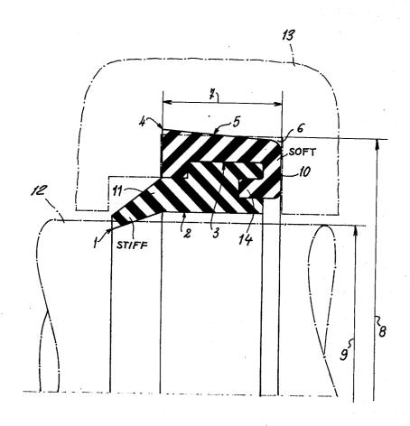
In accordance with yet another feature of this invention it is possible to use such a seal in a pneumatic cylinder or a low-pressure hydraulic cylinder.
