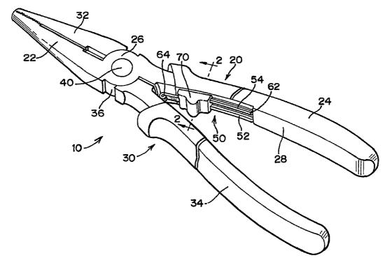
(57) **Abstract:** A hand tool (10) has two crossed members (20,30) each having a handle (24,34) and a jaw (22,32) connected to each other at a pivot point (26). A leaf spring (60) biases the handles (24,34) towards an open position. The leaf spring (60) can be selectively engaged or disengaged by the user by selectively moving a slider (70) over the spring (60).
