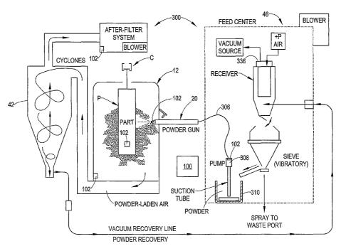
(57) Abstract: Material application system provided with a wireless identification technology for parts being processed and for components of the material application system. An exemplary technology is RFID. The RFID device can be used for many different functions including part identification, repair and maintenance programs, and inventory control.
