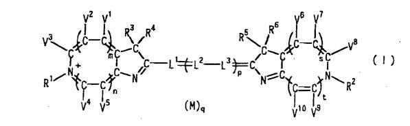
wherein R<sup>1</sup> and R<sup>2</sup> each independently represent an alkyl group that may be substituted with a reactive group capable of covalently bonding to A-B-; R<sup>3</sup>, R4, R<sup>5</sup>, and R<sup>6</sup> each independently represent an alkyl group, and R<sup>3</sup> and R<sup>4</sup>, and/
