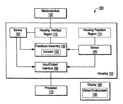
(57) Abstract: An apparatus comprises a manipulandum, a housing, a sensor and an actuator. The housing has a palpation region spaced apart from the manipulandum. The sensor is coupled to the palpation region of the housing. The sensor is configured to send a signal based on a palpation of the palpation region of the housing. The actuator is coupled to the manipulandum. The actuator is configured to send haptic output to the manipulandum based on the signal.
