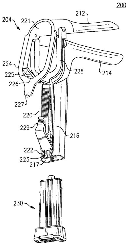
(57) Abstract: A vaginal speculum apparatus includes a disposable speculum and a releasably attachable illumination assembly. A handle portion of the disposable speculum includes a receiving cavity that is adapted to interchangeably receive either a first or a second illumination assembly.
