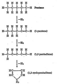
According to the invention, 1,3 pentadiene in 45 pure form, or admixed with normal pentane and/or normal pentenes, or other gases, is contacted with a mass consisting essentially of an alumina, which has been activated to yield a material having a highly porous adsorbent surface structure, at an elevated temperature for a time sufficient to effect a desired extent of conversion to 1,3 cyclopentadiene.
