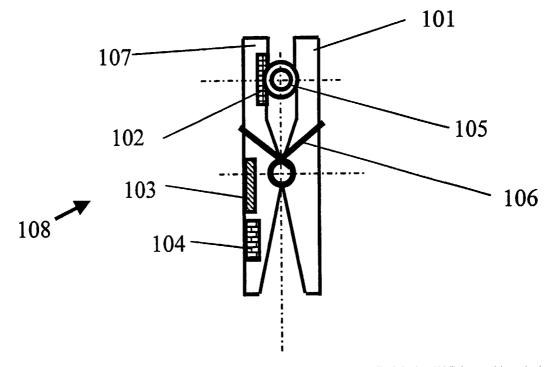
(57) Abstract: A method and apparatus for reducing morbidity associated with a medical device (105) inserted into the body of a patient. Ultrasonic energy is applied to the device with sufficient intensity to inhibit accretion of biological matter associated with the device while the device is in the body. Typically, the energy is applied to the device in the absence of clinically-observable accretion of biological matter on the device so as to prevent such accretion.
