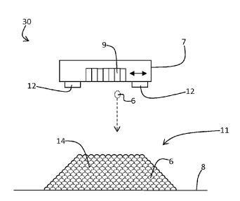
(57) Abstract: The present inventions refers to a method for printing an optical element (11) comprising the steps of ejecting at least one droplet (6) of printing material comprising silicone towards a substrate (8) in a first step and curing the droplet deposited on the substrate in a second step.
