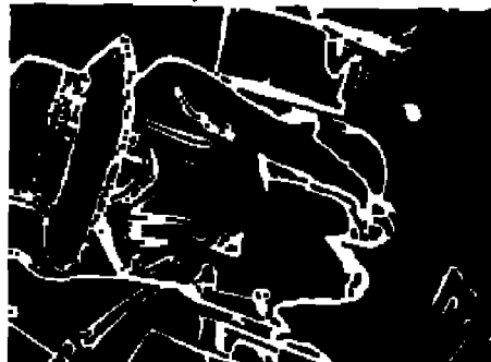
(6) Result from 3x3 Gaussian filter followed by max Kirsch filter, binarization, and morphological erosion.
