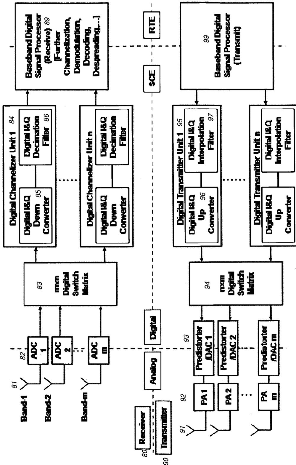
**FIG. 4. Digital-RF™ Multichannel Transceiver**
