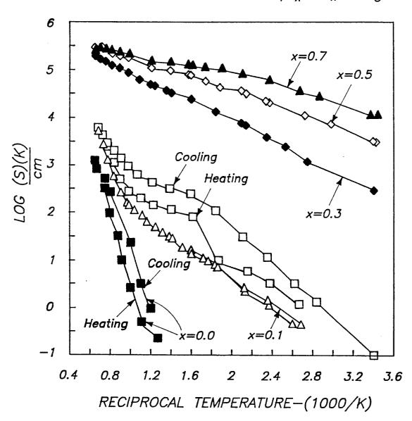
ELECTRICAL CONDUCTIVITY Y  $_{0.5}$  Ca  $_{0.5}$  MnO  $_{3}$  ; Y<sub>0.5</sub> Sr<sub>0.5</sub> MnO<sub>3</sub> AND La<sub>0.9</sub> Sr<sub>0.1</sub> MnO<sub>3</sub>
