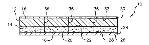
(57) Abstract: Improved binders, ink-receptive compositions, and coated substrates are provided. The ink-receptive compositions contain a binder, a particulate filler, and a mordant. A preferred binder comprises one or more acrylic copolymers made with at least one wet abrasion resistance-enhancing monomer. Papers, films, labels and similar products, coated with an ink-receptive composition, are also provided.
