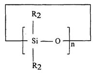
wherein  $R_1$  and  $R_2$  are independently selected from  $C_1$  to  $C_8$  alkyl, aryl or alkylaryl and wherein n=3-7. The linear polyorgano siloxanes have from about 2 to 7 silicon atoms and have the general formula:
